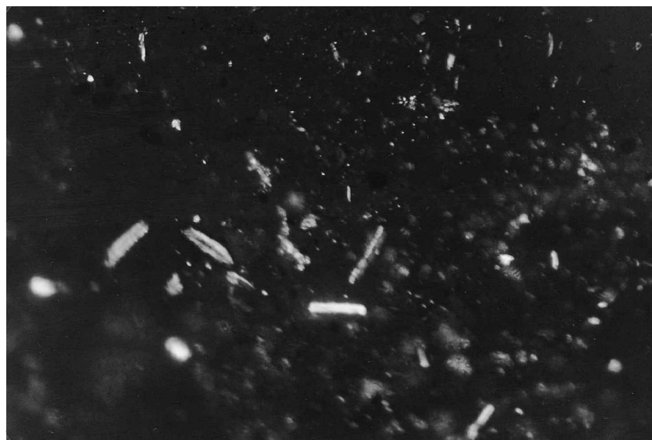
Figure 1. Polarizing photomicrograph of liquid crystalline acrylic copolymer GMBA4 at 25^{\circ}\text{C} .
